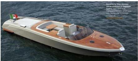
Newson's design for the Aquariva vessel is unique in its conception, as well as the materials chosen. A wood-like, textile-based laminate (phenolic composite) was used for the deck area and instrument panel. This material was developed in the first half of the 20th century, and was a precursor to fibreglass. While having an ostensibly organic feel and aesthetic, it is significantly more durable than wood.
